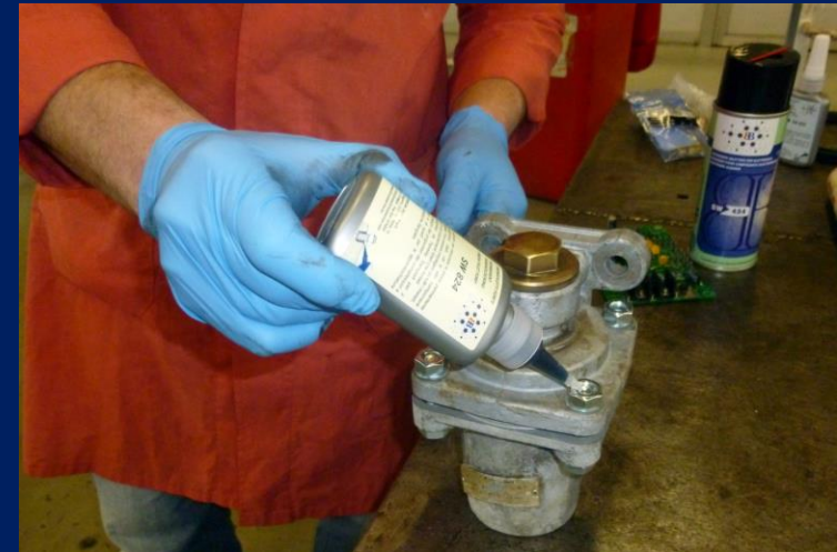
Threadlockers and fittings sealant approved by Faiveley Transport
