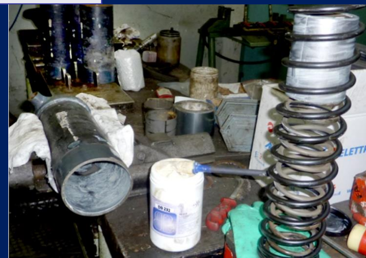
Cylindrical actuator of ETR 470 (tilting system component)
