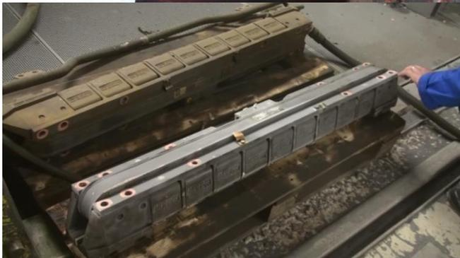
Compared to traditional methods the “cryogenic cleaning” allows the operator to reach hard to get to areas such as corners, crack where brushes or traditional abrasives can not get to. The dry ice pellets have weak cohesion. This means that it leaves the surfaces undamaged and leaves no wear or abrasion.
