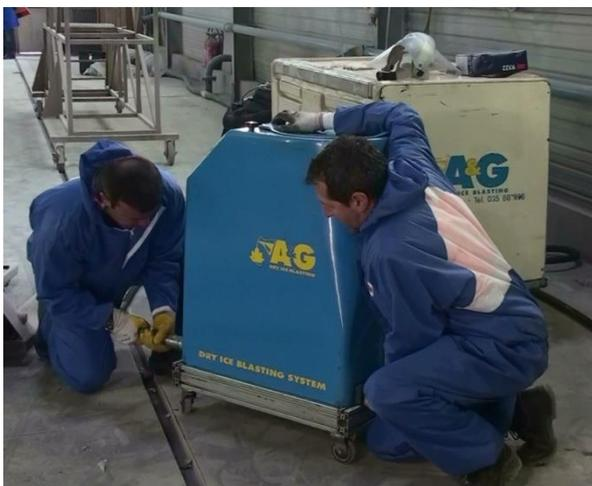
The special cleaning machine (**CO<sub>2</sub> accelerator - Dry ice blasting**),
