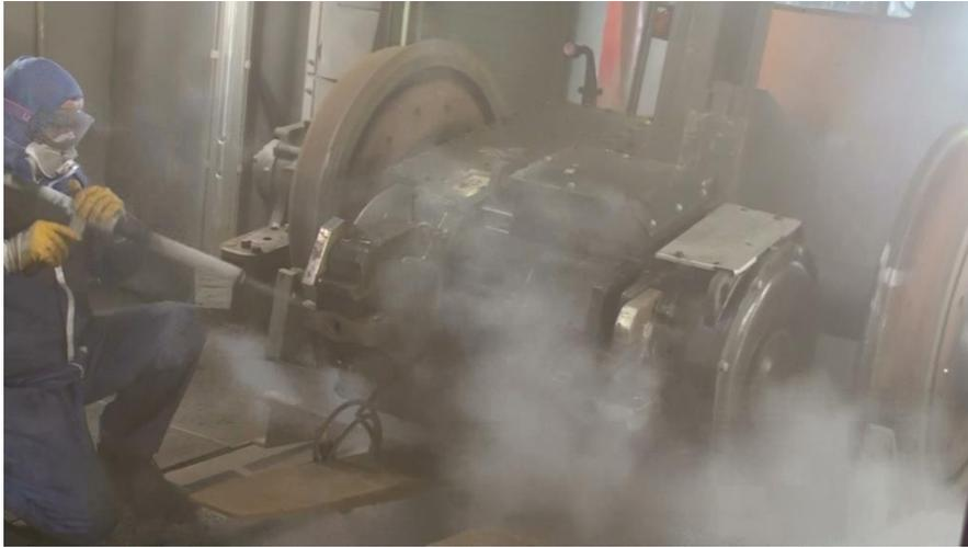
Cleaning with the CO<sub>2</sub> system permits the operator to do a visual analysis of the integrity of the components. From field trials the results have been very positive, analysis of various components shows no damage after the process, hence components that used the system were better than components that had not undergone the process. Essentially components cleaned with CO<sub>2</sub> have no drawbacks.
